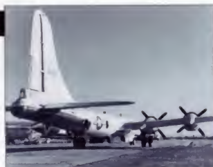
Above: Seen in February 1955, this WB-50D is one of 36 B-50D bombers stripped of weapons systems and used for weather reconnaissance. The last one was replaced by a WB-47 in 1967.
